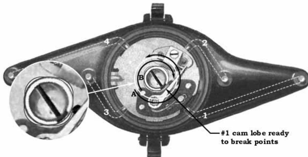
**A - Direction of rotation. Distributor cam in position to break the points for #1.**
